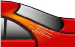
Mix Permasolid HS Race Clear Coat 8700, Permasolid Speed-TEC HS Speed Clear Coat 8810 or Permacron Rapidflex Clear Coat 8065 according to the TDS. Overcoat the chosen Spies Hecker basecoat quality with ready-to-spray clearcoat. Fade out the clearcoat in staggered coats with reduced pressure onto the sanded area and till the edge of the polished area.
