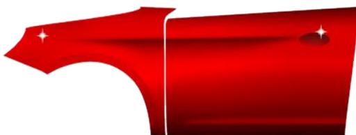
Another layer of the non-tinted clearcoat over the entire repair area is recommended to simplify the subsequent polishing work. Slower product adjustments, longer flash-off and drying times should be considered. Dry the clearcoat according to the technical data sheet. To improve the final topcoat appearance, this step can also be carried out after intermediate sanding with P1000.
