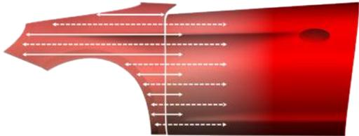
Blend-in and flash off the basecoat according to the TDS recommendations. Prepare the tinted clearcoat of the respective colour formulation according to the Phoenix colour software. Stir well immediately after addition of the Spies Hecker Clear Coat Color Additive. Prepare the same clearcoat non-tinted with the same hardener/reducer combination as the tinted clearcoat.
