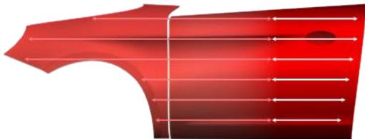
Use two spray guns or disposable cups in order to work quickly. Apply first coat of the tinted clearcoat to the repair part and extend into adjacent panel. Ensure that you spray over the edge of the previously applied basecoat colour. Straight after apply the first coat of the non-tinted clearcoat to the widest area of the adjacent panel and merge into the tinted clearcoat layer. Flash off.
