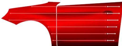
Apply second coat of the tinted clearcoat to repair part and extend into adjacent panel. Ensure that you spray over the edge of the first tinted clearcoat layer. Apply the second coat of the non-tinted clearcoat to the widest area of the adjacent panel and merge into the second coat of the tinted clearcoat.
