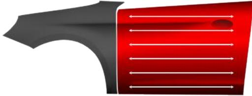
Repair panel: sand surfacer (minimum P500). Adjacent panel: prepare for blending with suitable abrasive e.g. Trizact – P1000.
