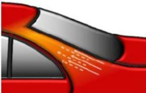
Mix any Permacron MS Clear Coat according to the TDS. Overcoat the Permacron Base Coat 293/295 with ready-to-spray Permacron MS Clear Coat. Fade-out the clear in staggered coats with reduced pressure within the sanded area.
