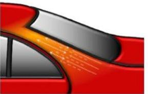
Mix Permacron Blend-In Reducer 1031 5:1 with the ready-to-spray Permacron MS Clear Coat and apply in thin coats with reduced pressure to the fade-out area. Dissolve the overspray and smooth the transition of the Permacron MS Clear Coat and stay within the P3000 sanded fade-out area.
