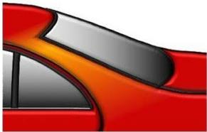
Sanding the fade-out area and the transition to the intact old paintwork, e.g. with 3M Trizact P3000 Fine Finishing Disc or similar abrasives from other suppliers.
