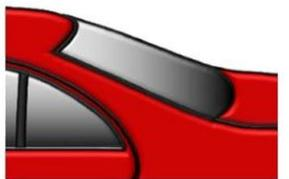
If required, lightly sand the transition zone after drying and cooling depending on the finish to be achieved e.g. with 3M Trizact P3000 or similar.
