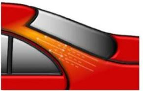
Mix Permacron Blend-In Reducer 1031 5:1 with the ready-to-spray Permacron Automotive Top Coat 257/MS, Automotive Top Coat 730 and apply in thin coats with reduced pressure to the fade-out area. Dissolve the overspray and smooth the transition of the Permacron Automotive Top Coat 257/MS, Automotive Top Coat 730 and stay within the P3000 sanded fade-out area.
