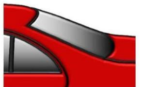
Mix the Permasolid HS Automotive Top Coat 275 according to the TDS. Apply the ready-to-spray Permasolid HS Automotive Top Coat 275 to cover the repair area and fade-out in staggered coats with reduced pressure within the sanded fade-out area.
