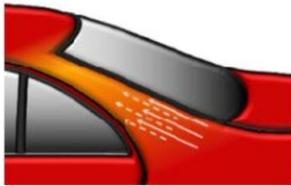
Mix the Permacron Automotive Top Coat 257/MS Automotive Top Coat 730 according to the TDS. Apply the ready-to-spray Permacron Automotive Top Coat 257/MS Automotive Top Coat 730 to cover the repair area and fade-out in staggered coats with reduced pressure within the sanded fade-out area.
