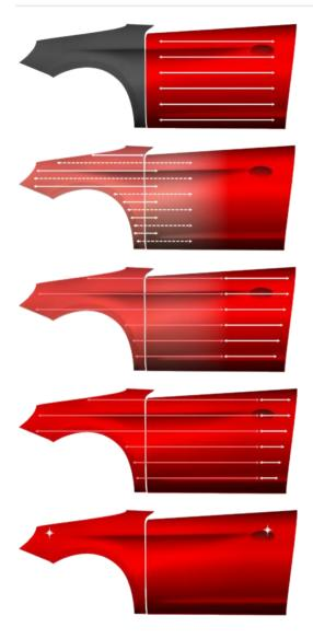
Repair panel: sand surfacer (minimum P500). Adjacent panel: prepare for blending with suitable abrasive e.g. Trizact – P1000.
