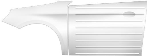
Apply a closed coat of hardened Permahyd Hi-TEC Blend-in Additive 1050/1051 (blender +5% Permahyd Hi-TEC Hardener 3080) to the adjacent blending area (panel). Do not fade out the blender and apply up to the edge of the panel.
