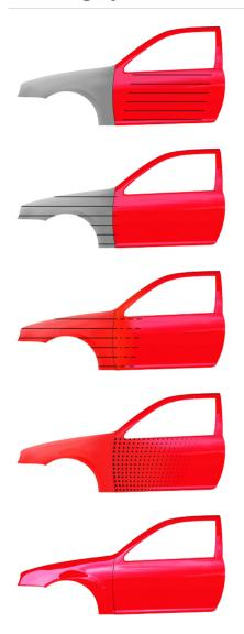
Apply one coat of Permacron 1K Clear Coat 8560 to adjacent panels or to the blending area around the spot repair. (This operation is optional )
