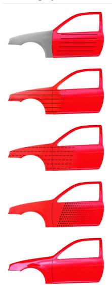
First apply one spray pass of Blend-In Additive 9005 to fade out area, but not up to undamaged edges of panels.\*
